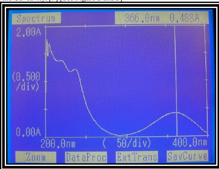
Figure 3: Photographic image showing \lambda_{\max} of felodipine after complexation (Figure 2 and 3 directly indicated increase in absorption maxima and bathochromic shift in \lambda_{\max} )
